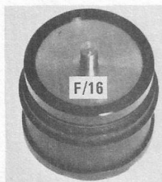
3650537 Use to set depth of inner and outer Helicoids.
