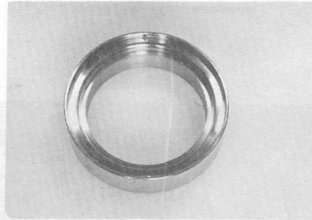
3650529 Use to remove/replace Diaphragm Ring Retainer O-M Mount.
